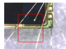
Damaged gold wire on an image sensor
